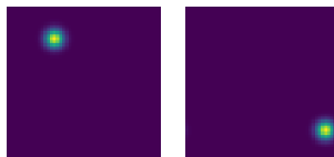
Figure 2. Display of the response of the operator E_{pq} to Dirac inputs x = \delta_u centered at two different locations u . These are bumps centered on points of the p - q diagonal, corresponding to interactions between two patches, at distance around p - q .
